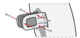
Position the assembly on the mast in the correct position and draw around the cheeks with a pencil.
