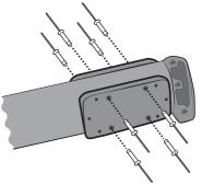
3. Make sure you have lined up the up the holes on the bracket, mounting plate and mast, run the 4mm drill bit through the holes, then attach the bracket using the 6 screws provided. Add a little Loctite to the threads of the screws first.
